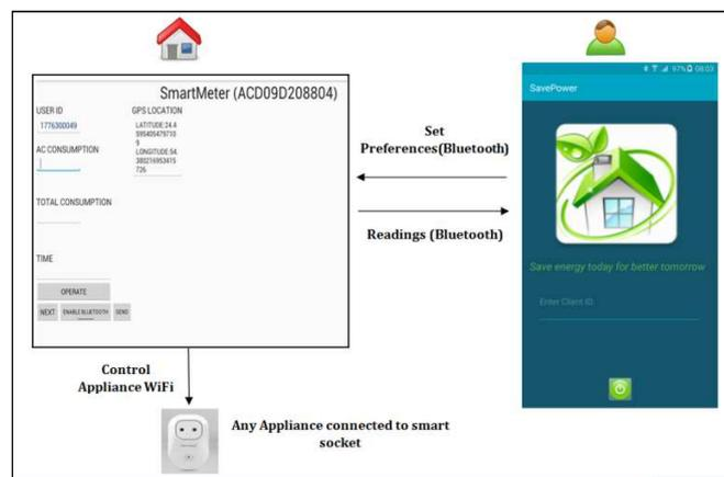
Fig. 5. Proposed Solution (Experimental Scenario) - *SavePower* hosts the control center unit database. *SmartMeter* has the GPS position the same as the consumer's household. *SmartMeter* hosts a temporary database for the specific consumer's household which is maintained for one day before being flushed with new readings.
