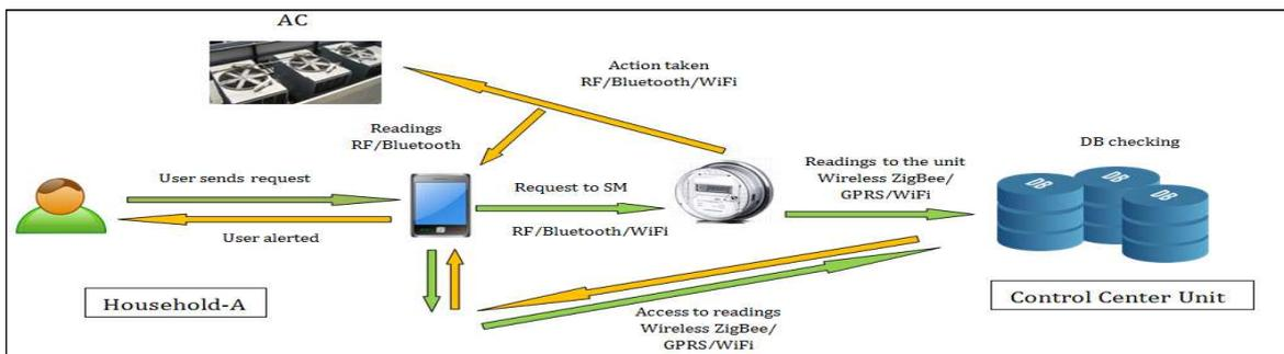
Fig. 3. Proposed Smartphone Application (Control Mode) - Consumers set their SM preferences using *SavePower* according to which SM controls AC. Preferences are sent via Bluetooth by *SavePower* and SM controls the AC via WiFi remotely. Criteria can be either GPS position or an overuse consumption threshold.
