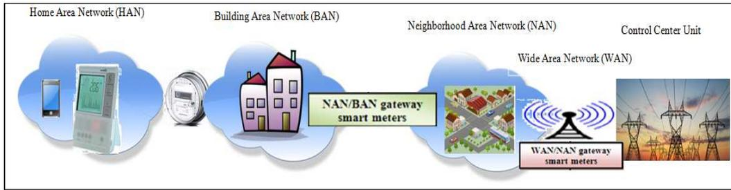
Fig. 2. Advanced Metering Infrastructure (AMI) - The proposed solution is located in HAN along with home appliances. SM works as a gateway to communicate electrical data consumption between *SavePower*, data concentrators in BAN and NAN, and the control center unit.
